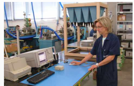
Final test with network analyzer
