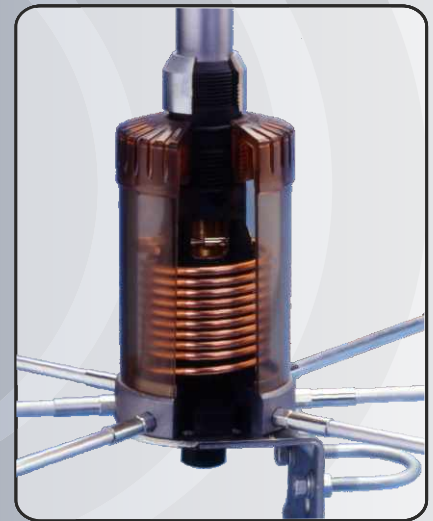
HI-Q LOW LOSS MATCHING COIL SUSPENDED ON 4 PLASTIC FINGER MADE OF COPPER WIRE \varnothing 4.5\text{mm} AWG-5
