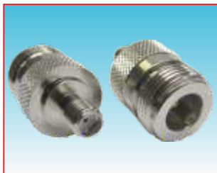
SMA-f / N-f adaptor Materials: Nickel plated brass, Delrin insulator, Gold plated central pin. P/N ..... 30.AD015.00
