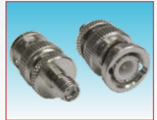
SMA-f / BNC-m adaptor Materials: Nickel plated brass, Delrin insulator, Gold plated central pin. P/N ..... 30.AD014.00
