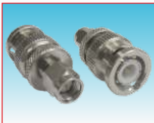
SMA-m / BNC-m adaptor Materials: Nickel plated brass, Delrin insulator, Gold plated central pin. P/N ..... 30.AD019.00
