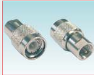
FME-m / TNC-m adaptor Materials: Nickel plated brass, Delrin insulator, Gold plated central pin. P/N ..... 30.AD003.00
