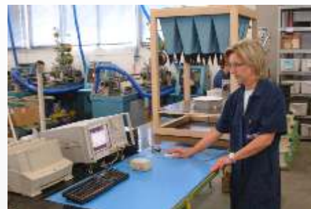
Final test with network analyzer
