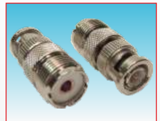
UHF-f / BNC-m adaptor Materials: Nickel plated brass, Delrin insulator, Gold plated central pin. P/N ..... 30.AD022.00
