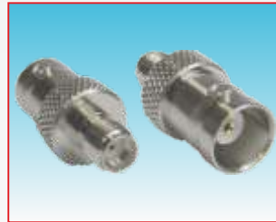
SMA-f / BNC-f adaptor Materials: Nickel plated brass, Delrin insulator, Gold plated central pin. P/N ..... 30.AD013.00
