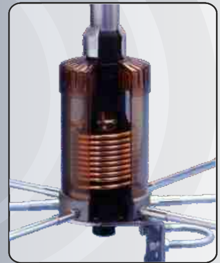
HI-Q LOW LOSS MATCHING COIL SUSPENDED ON 4 PLASTIC FINGER MADE OF COPPER WIRE \varnothing 4.5mm AWG-5
